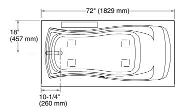
No change in measurements if connected with drain illustrated. (K-7166-AF)
