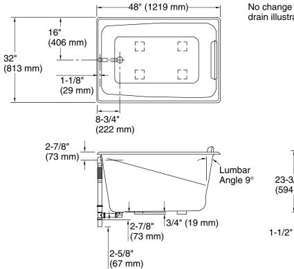
No change in measurement if connected with drain illustrated. (K-7265)
