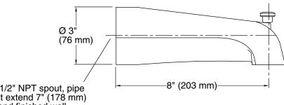
For 1/2" NPT spout, pipe must extend 7" (178 mm) beyond finished wall.
