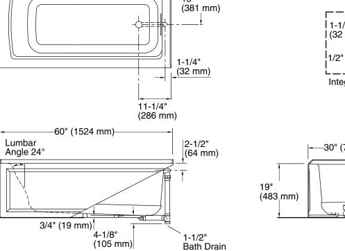
No change in measurements if connected
