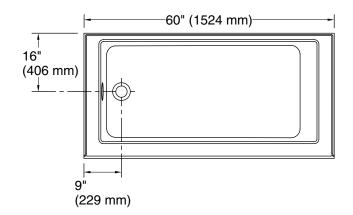
No change in measurements if connected with drain illustrated. (K-7259)
