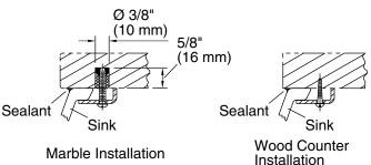
Note: Waterproof unprotected overhang area on the underside of wood counter.
