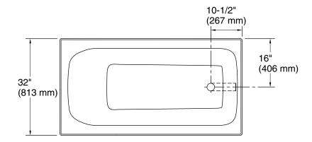
No change in measurements if connected with drain illustrated. (1381626)
