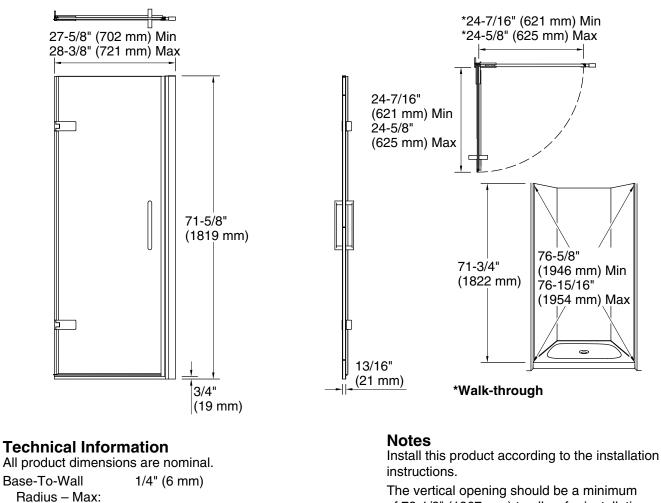
The vertical opening should be a minimum of 73-1/2" (1867 mm) to allow for installation clearance.
