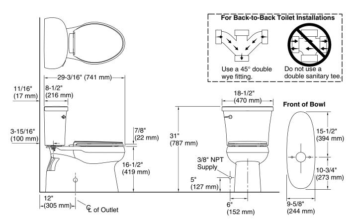
**Technical Information** All product dimensions are nominal. Toilet type: Floor-mount Waste Outlet: Floor Bowl shape: Elongated **Class Five** Flush type: 2-1/8" (54 mm) Trap passageway: 9-3/4" x 6-7/8" (248 mm x 174 mm) Water surface size: Rim to water 5-7/8" (149 mm) surface: Rough-in: 12" (305 mm) Seat-mounting 5-1/2" (140 mm) holes:
