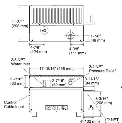
Minimum required access panel is 24" (610 mm) L x 15" (381 mm) H.
