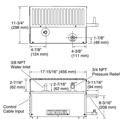
Minimum required access panel is 24" (610 mm) L x 15" (381 mm) H.
