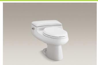
The Comfort Height® one-piece toilet shall be made of vitreous china and 1.0 gpf (3.8 lpf). Toilet shall be 30" (762 mm) in length, 19-1/2" (495 mm) in width, and 21-1/2" (546 mm) in height. Toilet shall have a 9" (229 mm) x 7" (178 mm) water area, and a 12" (305 mm) rough-in. Toilet shall be equipped with Sloan Flushmate® Pressure Vessel. Toilet shall include seat and cover. Toilet shall be less supply.
