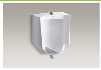
Urinal shall be 26-7/8" (683 mm) in height, 18" (457 mm) in width, and 14-1/8" (359 mm) in depth. Urinal shall be made of vitreous china. Urinal shall have washout flushing action. Urinal shall have 3/4" top spud and 14-1/8" (359 mm) extended rim. Urinal shall use 0.125 gpf (0.47 lpf) to 1.0 gpf (3.8 lpf) depending on flushometer specified. Urinal shall be WaterSensecompliant when used with a WaterSense flushometer. Urinal shall be K-4904-ET.
