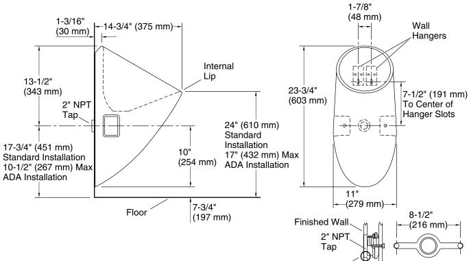
Finished wall and back of spud should be flush. Outlet Detail
