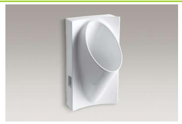
The waterless urinal shall be constructed of vitreous china. Urinal shall be 29-5/8" in height, 15" in width, and 15-5/8" in depth. Urinal shall have cartridge-free waterless functionality. Internal trapway shall provide enhanced performance and less maintenance. Urinal shall have optimized desing to virtually eliminate splashing. Urinal shall have a touch-free design offering vandal resistance and added hygiene to users.
