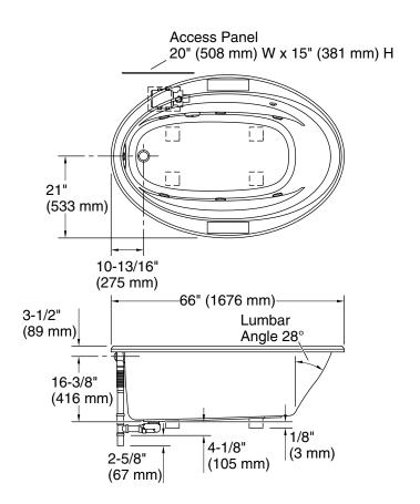
No change in measurements if connected with drain illustrated. (K-37382)
