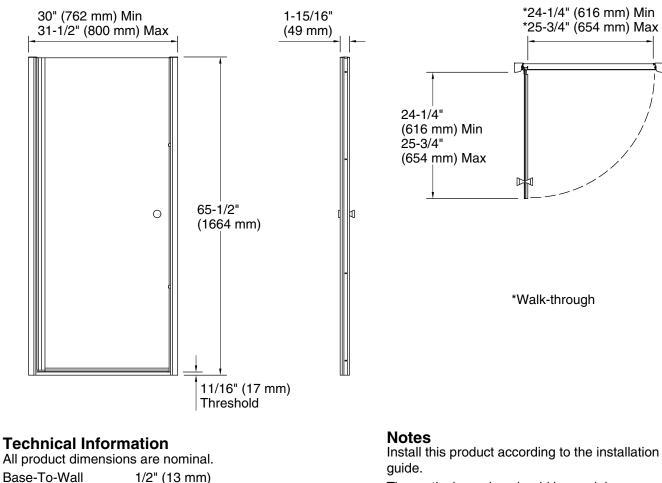
The vertical opening should be a minimum of 66" (1676 mm) to allow for installation clearance.
