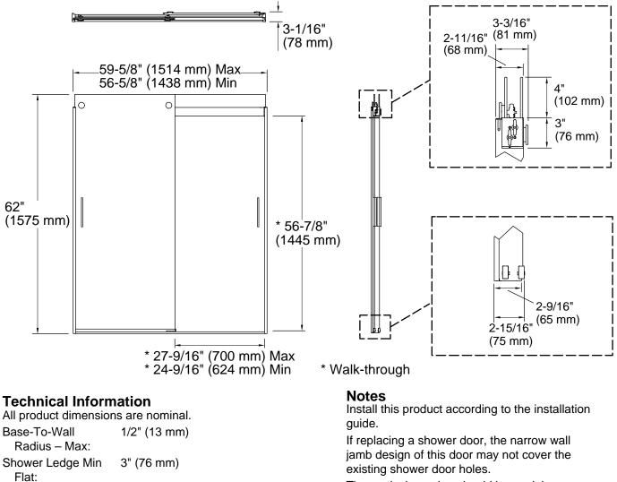
The vertical opening should be a minimum of 64-1/2" (1638 mm) to allow for installation clearance.
