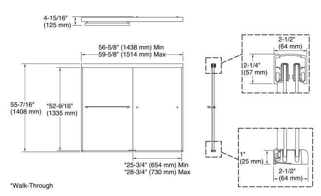
Technical InformationAll product dimensions are nominal.Base-To-Wall3/8" (10 mm)Radius – Max:3/8" (10 mm)Shower Ledge Min2-1/2" (64 mm)Flat:2-1/2" (64 mm)Flat:2-1/2" (64 mm)
