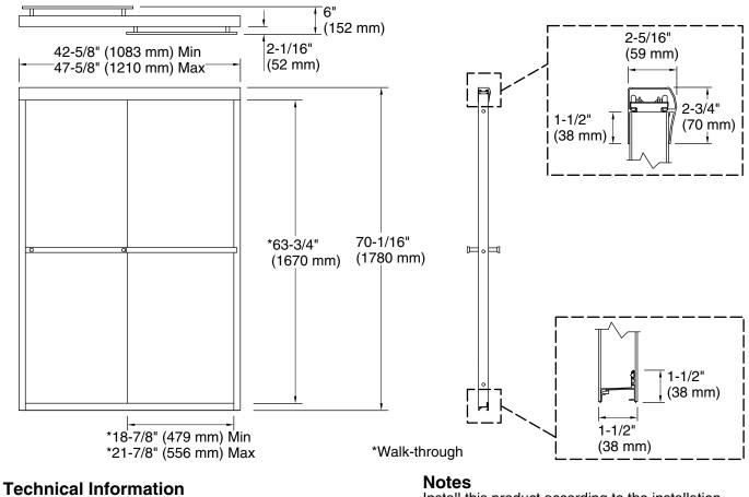
All product dimensions are nominal. Base-To-Wall 5/8" (16 mm) Radius – Max: Install this product according to the installation instructions.
