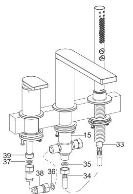
Put the washer(35) into the nut of the hose(34). Connect the connection hose to the diverter kit(15).
