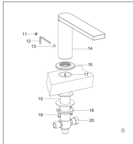
Slide the o-ring(17) into the bottom groove of the escutcheon(16). Tighten the escutcheon with the o-ring onto the diverter kit(15), and keep it against the bath tub. Position the diverter kit so that the nut(20) is on the right. Screw the nut(18). Tighten the screws(19) to secure the diverter kit.
