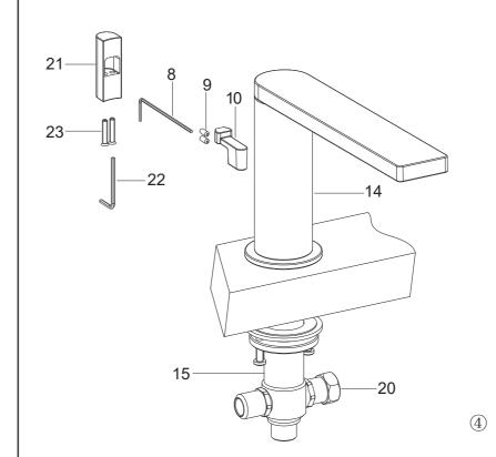
Install the connector(10) to the diverter kit.
