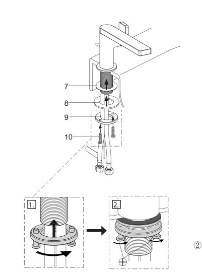
Position the faucet, install the screws(10) into the mounting nut(9). From underside of the lavatory, place the washers(7, 8) onto the shank. Tighten the mounting nut to secure the faucet. Tighten the screw.
