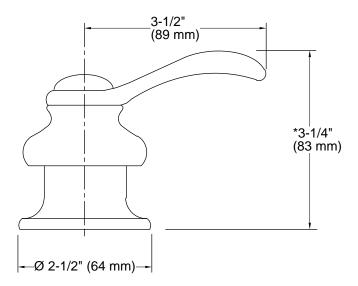
\* Allows for +/- 1/4" (6 mm) handle adjustment.
