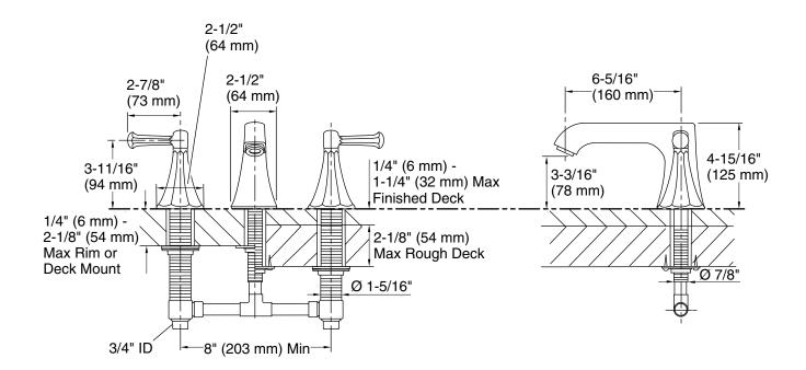
Rim- or Deck-Mount Installation Rough + Finished Deck-Mount Installation
