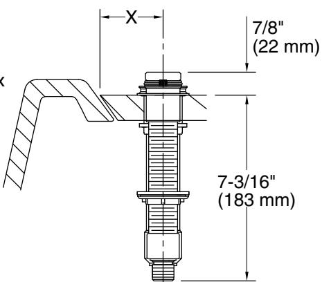
X = Distance from centerline of spout inlet to front of spout base plus 1/2" (13 mm).
