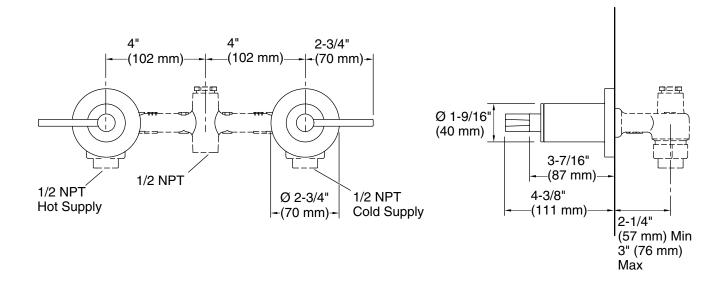
Technical Information All product dimensions are nominal. Drain included: No Notes ADA, OBC, CSA B651 compliant when installed to the specific requirements of these regulations.
