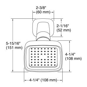
Technical Information All product dimensions are nominal. Drain included: No Shower/Rainhead rated max 1.75 gal/min (6.6 l/min) flow: Notes Install this product according to the installation instructions.
