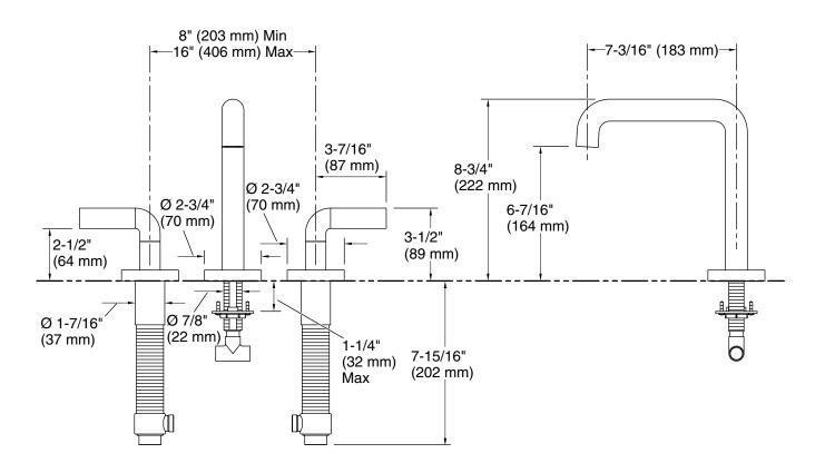
**Technical Information** All product dimensions are nominal. Faucet flow rate: 8 gal/min (30.3 l/min) Drain included: No Drain with No these regulations. overflow:
