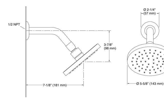
Technical Information All product dimensions are nominal. Drain included: No Shower/Rainhead rated max 1.75 gal/min (6.6 l/min) flow: Notes Install this product according to the installation instructions.
