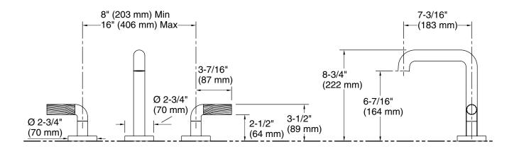
Technical Information<br/>All product dimensions are nominal.Notes<br/>Install this product according to the<br/>installation instructions.Faucet flow rate:9.98 gal/min (37.8 l/min)Drain included:NoSpout:7-3/16" (183 mm)
