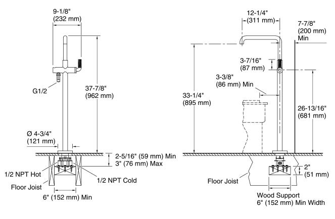
Technical InformationAll product dimensions are nominal.Faucet flow rate:8 gal/min (30.3 l/min)Drain included:NoSpout:Spout reach:12-1/4" (311 mm)Handle clearance:3-7/16" (87 mm)
