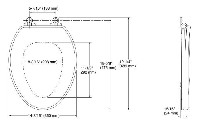
Technical InformationAll product dimensions are nominal.Seat shape type:ElongatedSeat front type:Closed-frontSeat hinge type:CheckSeat-mounting5-1/2" (140 mm)holes:Check
