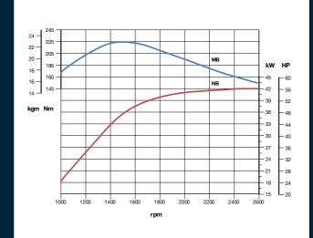
MB – Torque curve NB – Power curve
