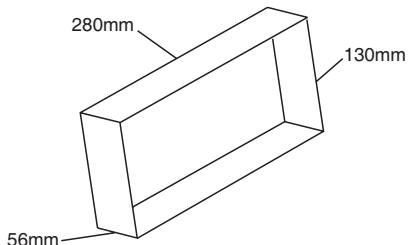
2. Put the tissue box into the groove and then mark the four installation holes.
