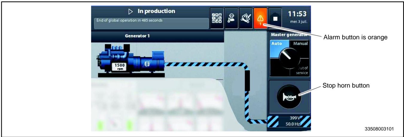
Figure 38 Appearance of an Alarm (warning)
