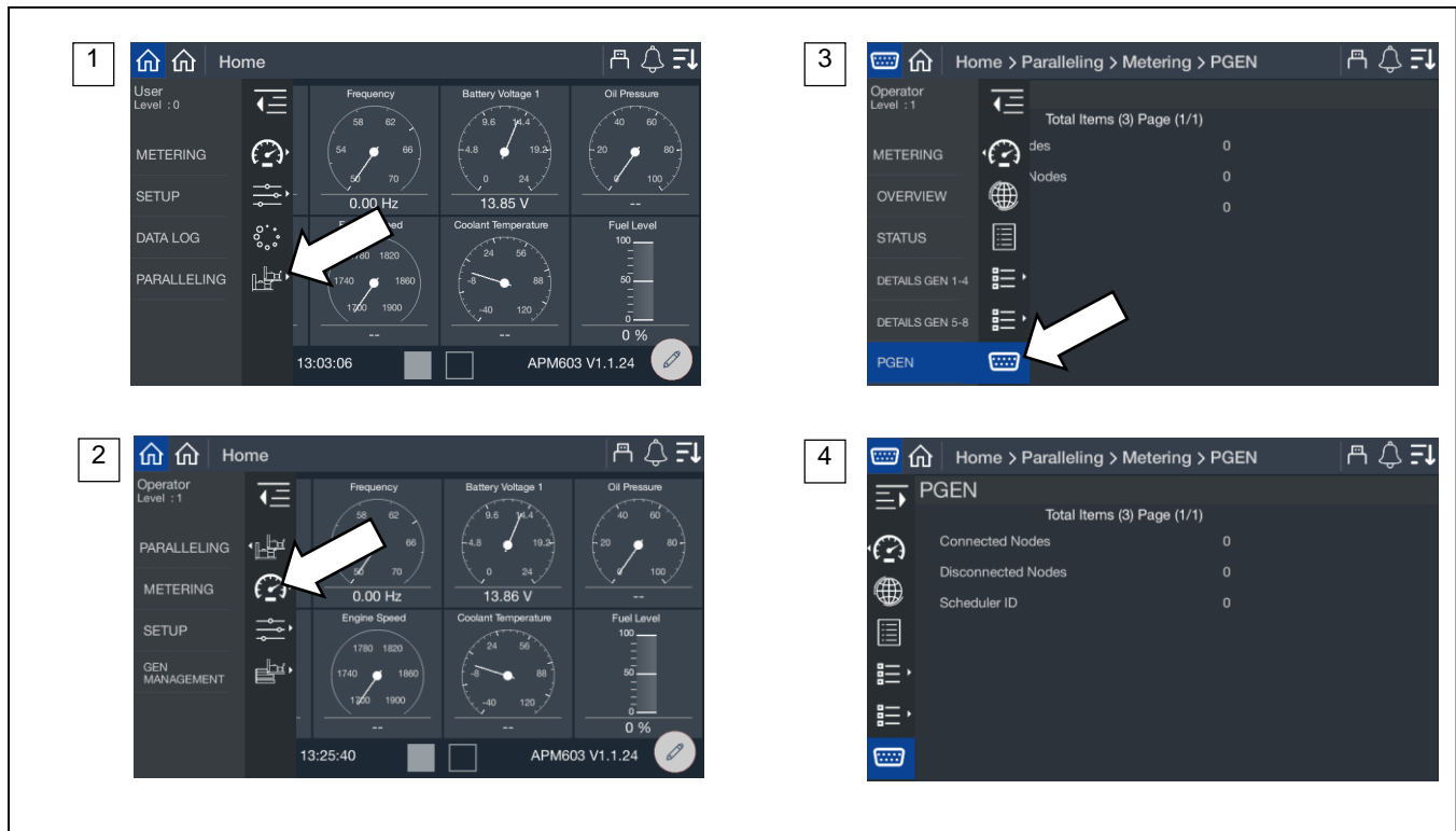
Figure 64 Paralleling, Metering, PGEN
