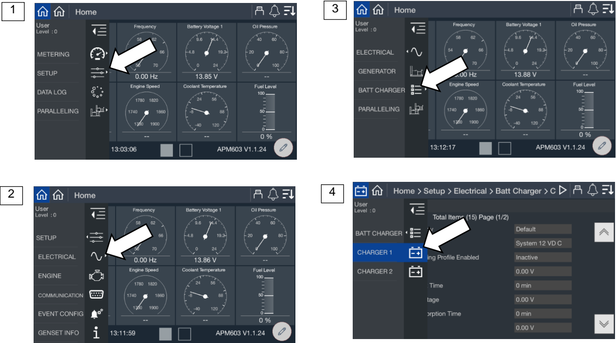
Figure 46 Battery Charger Setup Screen
